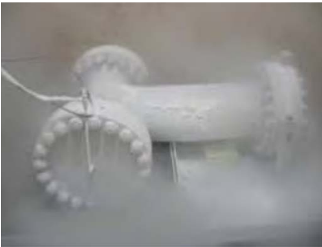
Tee body basket strainer following emissions test at -140°C
