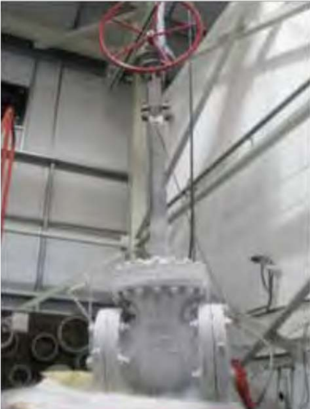
10" 300RF BS6364 cold box extended bonnet gate valve following test at -196°C
